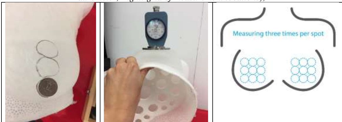
Figure 11. Durometer Technique (Left: location placement, Middle: torso tilting for normal durometer, Right: grid of measurement locations);
