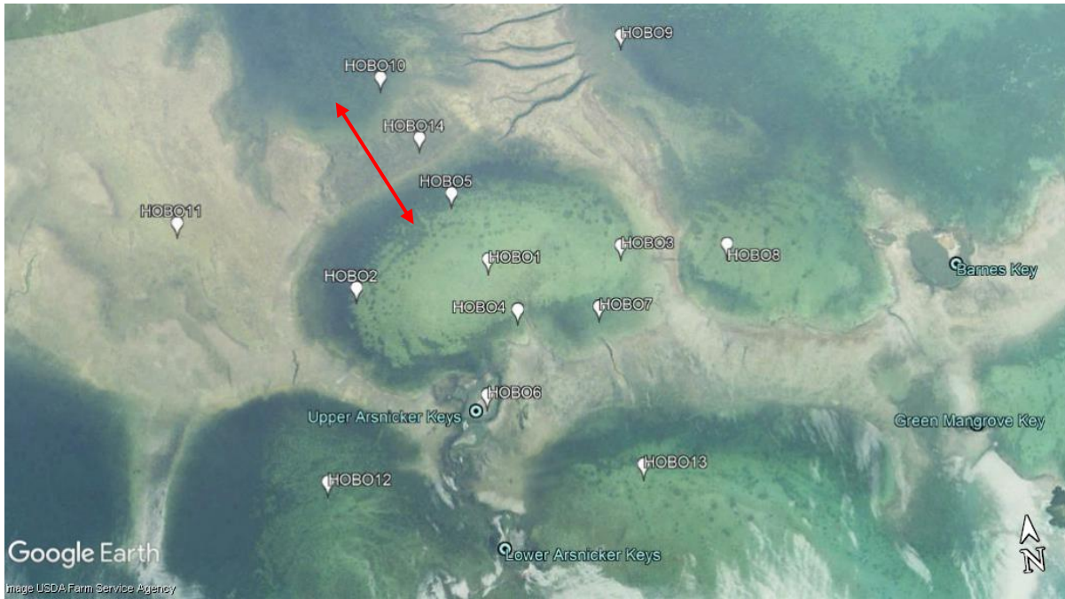
Figure 1 Satellite image of Mystery Basin and surrounding basins. HOBOL1 is the center of the basin and the location of one of the Onset pressure sensors and the in-situ sensor array. The other HOBOL pressure sensor locations are shown as well, numbering 1 to 14. Red arrow indicates predominant direction of water exchange in and out of MB.
