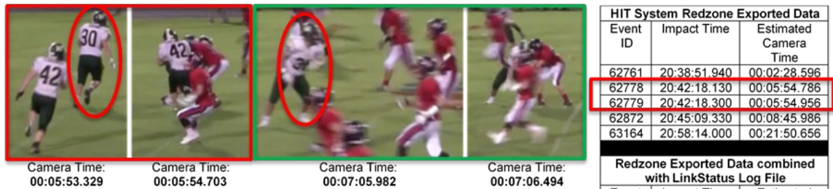
Figure 2.5: Example of the HIT System misclassifying a true head impact. The HIT system uses proprietary algorithms to provide users with clean datasets through their Redzone cloud-based software. However, impacts are removed from the Redzone exported data that could be relevant to injury risk. The player circled in red experienced a concussion in this game. The figure boxed in red shows an impact captured through video that corresponded to the HIT System Redzone exported data boxed in red on the right. Just over a minute later the same player sustained an impact (image in green) that lead to removal from the game. No data from the Redzone export corresponded to this impact with the closest time stamp occurring 3 minutes after the impact in red. Extracting data from the LinkStatus Log file showed that the HIT system triggered during the impact in green and corresponded to an impact time (green box on right) occurring a minute after the impact in red. Unfortunately, the algorithm filtered this data from the Redzone data export.
