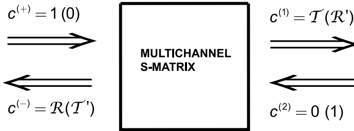
Fig. 2. Computation of the elements of the multichannel S-matrix in terms of reflection and transmission coefficients. The coefficients \mathcal{T} and \mathcal{R} are associated with transmission and reflection by the “black box” or transitional domain, as caused by the generic interaction, for right movers—they determine the first column of the S-matrix. Likewise, the coefficients \mathcal{T}' and \mathcal{R}' are associated with left movers (in parentheses)—they determine the second column of the S-matrix. The double arrows indicate that the attached labels are amplitude coefficients (as opposed to the single arrows of Fig. 1 representing basis functions).
