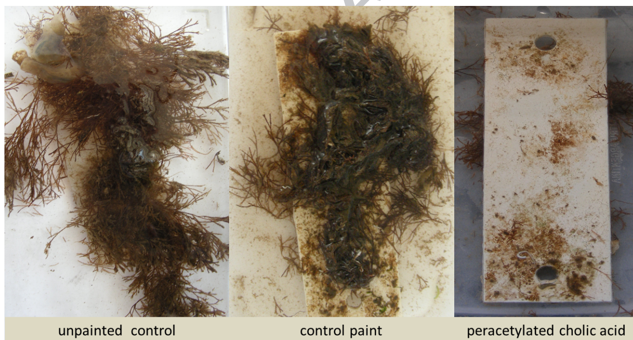
Fig. 6 Settlement on panels after 90 days exposure.
