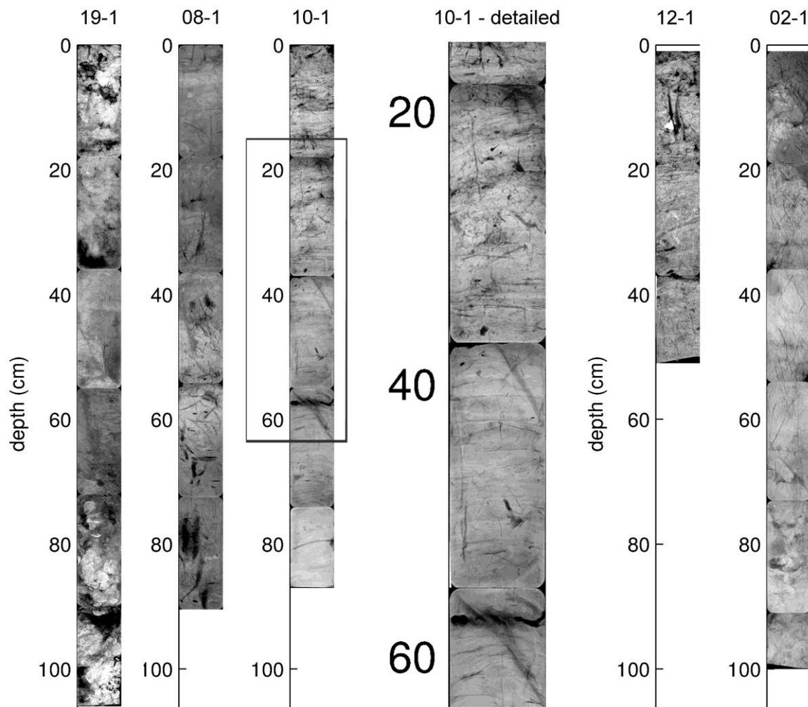
Figure 5: X-ray radiographies of the cores that have been dated by means of radioisotope analysis. Additionally, a detailed view on the transition zone from tidal flat to salt marsh in core 10-1 is shown in panel 4.
