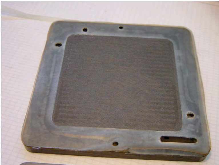
Figure 12. Cell # 5 gasket and diffusion layer which showed no degradation
