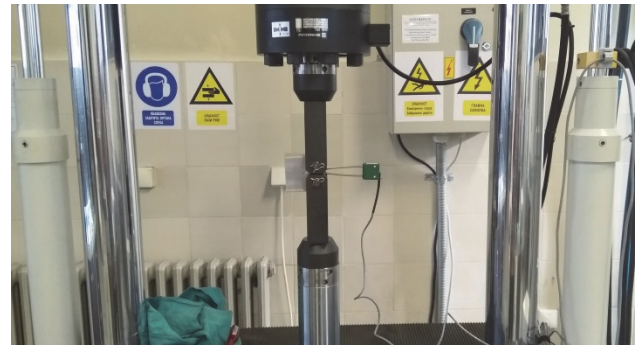
Figure 3 Test specimen fixed between the clamping heads of the SHIMADZU ServoPulser E-type servo-hydraulic test machine, with extensometer
