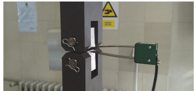
Figure 4 Installation of extensometer
