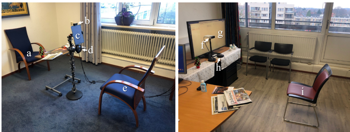
Figure 2: Rooms and set up of the experiment. On the resident's side (left): a = chair onto which the family member would be projected; b = Logitech webcam; c = iPad; d = Jabra 750 speakerphone; e = position of the resident. On the family member's side (right): f = Azure Kinect camera; g = TV screen; h = Jabra 750 speakerphone; i = position of the family member.
