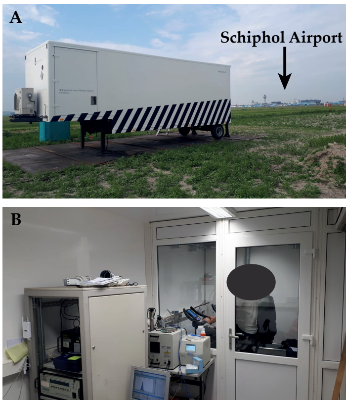
Figure 1. Exposures were conducted in an exposure laboratory right next to Schiphol Airport (A). It consisted of two chambers: one chamber in which subjects were exposed and one for the exposure monitoring equipment (B).
