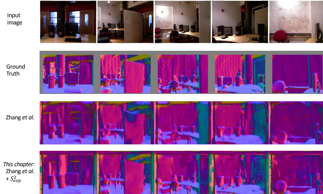
FIGURE A.2: Visualization of Surface Normal Estimation on NYU v2. Predictions are made by model: “Zhang et al. [179]” and “Zhang et al. [179] + S^2_{exp} ”. While results from Zhang et al. [179] are smoother, our method generates sharp boundaries and thus maintains details.
