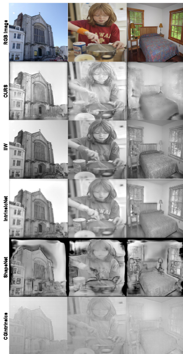
Fig. 11. Shading evaluations on IIW. Our model can produce scene-level shading maps that are free of texture or intensity ambiguities. Other models tend to overfit to the RGB images. (For interpretation of the references to color in this figure legend, the reader is referred to the web version of this article.)
