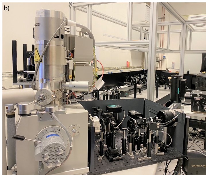
Figure 3.1: Pump-probe cathodoluminescence setup. Schematic (a) and photograph (b) of our PP-CL setup. The setup consists of the electron (purple), light-injection (green) and collection (orange) paths. The fundamental output ( \lambda = 1035 \text{ nm} ) of a femtosecond laser is converted to the 2 nd , 3 rd and 4 th harmonics ( \lambda = 517, 345 and 258 \text{ nm} , respectively) in the harmonic generator (HG) setup. The 4 th harmonic is focused on the electron cathode of the SEM to generate electron pulses. The 2 nd or 3 rd harmonics are directed towards the SEM chamber using either a beam splitter or dichroic mirror (BS, DM) to optically excite the sample. The delay between electron and light pulses is controlled using two delay lines (DL1 and DL2). The alignment between the air-suspended parts and the optical table is maintained using a feedback system (FS).
