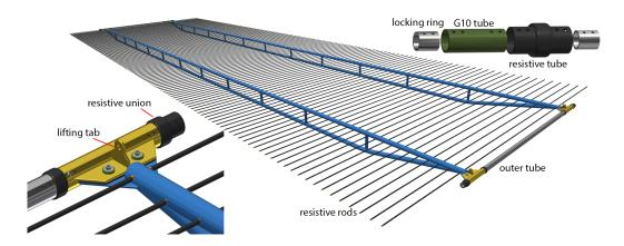
**Figure 4.4.** Illustration of a DP cathode module. It is constructed using a pair of stainless steel trusses (blue) as the framework with an array of coated FRP rods. The lower-left inset shows the resistive interconnections and the lifting tab on the cathode truss structure. The upper-right inset is shows the resistive union.
