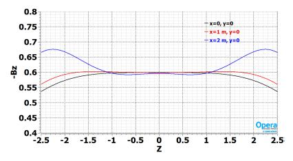
**Figure A.25**. Field map of the superconducting magnet along the z axis. The colors represent different radii from the center line.
