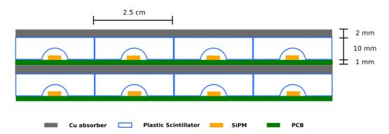
**Figure A.23**. Conceptual layout of the ECAL showing the absorber structure, scintillator tiles, SiPMs and PCB.
