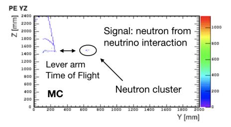
**Figure A.44**. An example of the antineutrino interaction in a 2.4×2.4×2.0 m<sup>3</sup> 3DST. The number of photoelectrons (PE) is plotted. An isolated cluster of hits corresponds to a neutron indirect signature produced by the antineutrino interaction.
