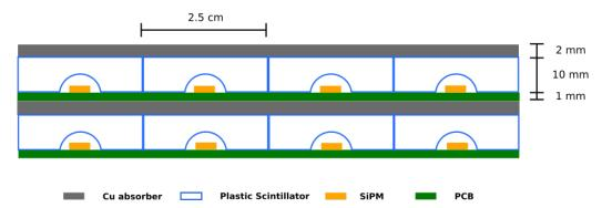
**Figure 5.3**. Conceptual layout of the calorimeter showing the absorber structure, scintillator tiles, SiPMs, and PCB. The scintillating layers consist of a mix of tiles and cross-strips with embedded wavelength shifting fibers to achieve a comparable effective granularity.
