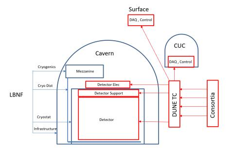
**Figure 7.9**. Overall integration nodes and interfaces. The items provided by LBNF within the cavern are shown on the left and the items provided by DUNE are on the right.
