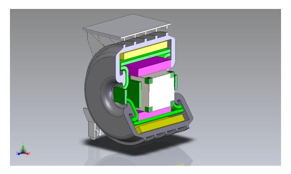
**Figure A.40**. The 3DST inside the KLOE magnet. The drawing shows the 3DST in the center (white), TPCs (orange), ECAL (green), magnet coil (yellow), and the return yoke (gray).
