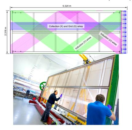
**Figure 3.2**. Top: a schematic of an APA. The steel APA frame is shown in black. The green and magenta lines indicate the directions of the induction wire layers. The blue lines indicate the directions of the induction and shielding (grid) wire layers. The blue boxes at the right end are the CE. Bottom: a ProtoDUNE-SP APA in a wire-winding machine. The end on the right is the head end, onto which the CE are mounted.
