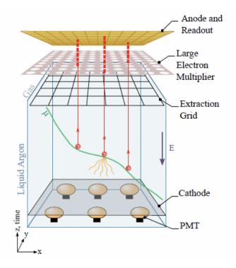
**Figure 4.1**. Principle of the DP readout.
