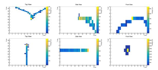
**Figure A.42**. Event displays showing the three two-dimensional projections of energy from a photon conversion (top) and a stopping proton (bottom). From data collected at the 2018 test beams at the CERN T9 area.
