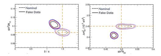
**Figure A.34**. The results of a full two-flavor, antineutrino+neutrino, near+far oscillation fit are shown for a fit to the nominal MC (dashed) and a fit to the fake data set (solid). The true values of the oscillation parameters in each of the data sets are indicated by the dashed yellow lines. Clear biases can be see in all oscillation parameters that are well outside the  $1\sigma$  (black),  $2\sigma$  (red), and  $3\sigma$  (blue) contours.
