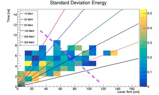
**Figure A.48**. Energy resolution of the neutron candidates in the (time, lever arm) space. The dashed line corresponds to the cut required to select an almost 100% pure sample of signal neutrons. The solid lines are theoretical curves for neutrons with different kinetic energies. Note that this study was performed with a total volume of  $2.0\times2.0\times2.0 \,\mathrm{m}^3$ . See text for details.
