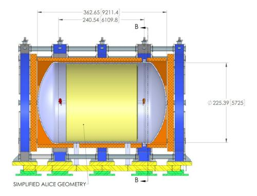
**Figure 5.2**. The conceptual design of the MPD system for the ND. The TPC is shown in yellow inside the pressure vessel. Outside the pressure vessel, the ECAL is shown in orange, and outside that are the magnet coils and cryostats. The drawing illustrates the five-coil superconducting design.
