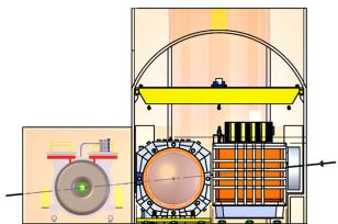
**Figure B.1**. DUNE ND hall shown from above (top) and from the side transverse to the beam (bottom). The LArTPC, MPD, and 3DST detectors are shown in position on the beam axis in both drawings.
