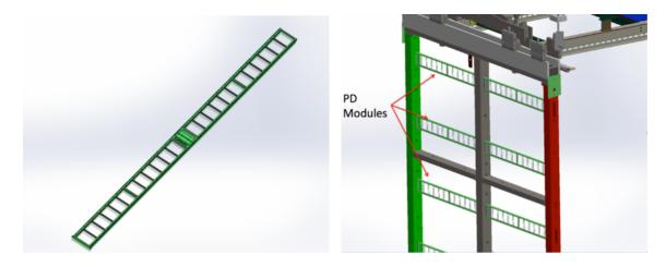
**Figure 3.6**. Left: an X-ARAPUCA PD module. The 48 SiPMs that detect the light from the 24 cells are along the long edges of the module. Right: X-ARAPUCA PD modules mounted inside an APA.
