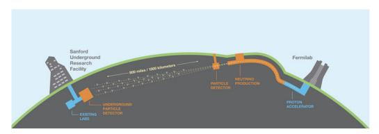
**Figure 1.1**. Cartoon illustrating the configuration of the LBNF beamline at Fermilab, in Illinois, and the DUNE detectors in Illinois and South Dakota, separated by 1300 km.
