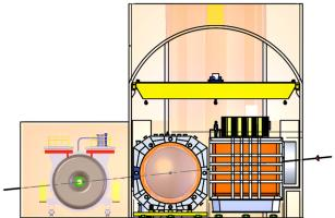
**Figure 5.7**. DUNE ND hall shown from above (top) and from the side transverse to the beam (bottom). The ArgonCube, MPD, and SAND are shown (in that order, bottom to top, in the upper figure) in position on the beam axis (black arrow) in both drawings.
