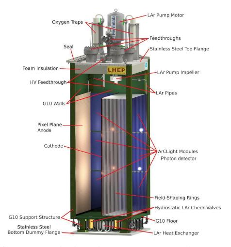
**Figure A.4.** Cutaway drawing of a  $0.67 \,\mathrm{m} \times 0.67 \,\mathrm{m} \times 1.81 \,\mathrm{m}$  ArgonCube module for the  $2\times2$  demonstrator module. For illustrative purposes the drawing shows traditional field-shaping rings instead of a resistive field shell. The G10 walls will completely seal the module, isolating it from the neighboring modules and the outer LAr bath. The  $2\times2$  modules will not have individual pumps and filters.
