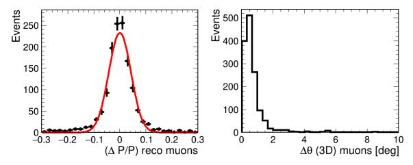
**Figure A.31**. Left: the momentum resolution for reconstructed muons in GArSoft, in a sample of 2 GeV  $\nu_{\mu}$  CC events simulated with GENIE. The Gaussian fit to the  $\Delta p/p$  distribution has a width of 4.2%. Right: the 3D angular resolution for the same sample of muons in GArSoft.
