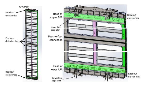
**Figure 3.3**. Left: two vertically linked APAs form one unit of an APA array. PD bars are installed across the width of the APAs. Right: a zoom into only the top and bottom ends of the APA stack (notice the breaks in white). This shows the readout electronics and the center of the stack where the APAs are connected.
