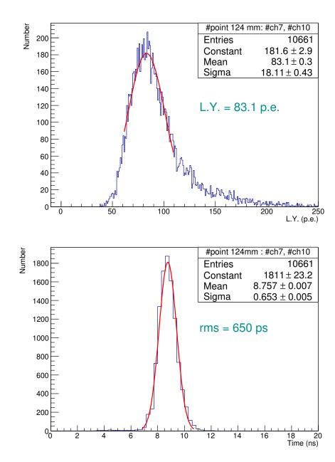
**Figure A.41**. Charge and time spectra for a single 3DST cube. Charge signal is a sum from two fibers, the time is an average time between two fibers.
