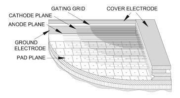
Figure A.20. Schematic diagram of the ALICE MWPC-based ROC with pad plane readout, from ref. [112].
