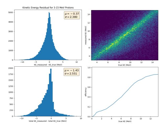
**Figure A.32**. (Top left) Kinetic energy residual, (Top right) measured KE vs. true KE, and (Bottom right) reconstruction efficiency for individual protons with 3 MeV to 15 MeV KE in the test set. (Bottom left) Residual of the total kinetic energy of all protons in each event in the test sample.
