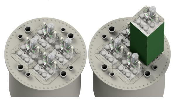
**Figure A.3**. Illustration of the ArgonCube 2×2 demonstrator module. The four modules are visible, with one of them partly extracted, on the right. This figure has been reproduced from ref. [89].
