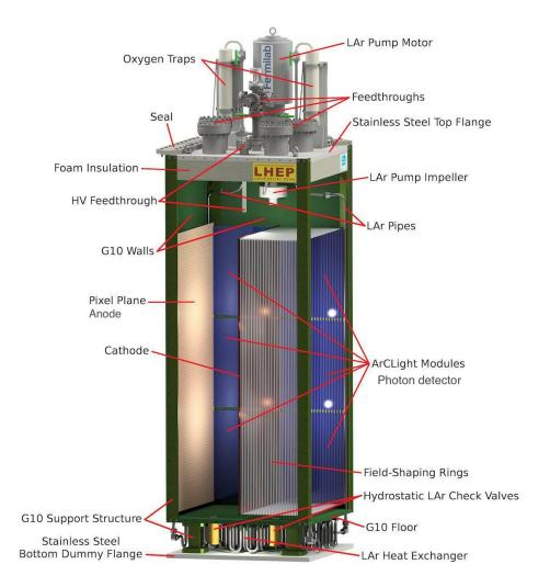
**Figure 5.1.** Cutaway drawing of a  $0.67 \, \text{m} \times 0.67 \, \text{m} \times 1.81 \, \text{m}$  ArgonCube prototype module. For illustrative purposes, the drawing shows traditional field-shaping rings instead of a resistive field shell. The G10 walls will completely seal the module, isolating it from the neighboring modules and the outer LAr bath. The modules in this prototype system will not have individual pumps and filters.
