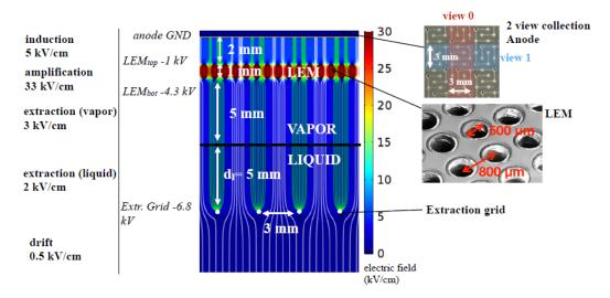
**Figure 4.3**. Thicknesses and HV values for electron extraction from liquid to gaseous argon, their multiplication by LEMs, and their collection on the x and y readout anode plane. The HV values are indicated for a drift field of  $0.5 \, \text{kV/cm}$  in LAr.
