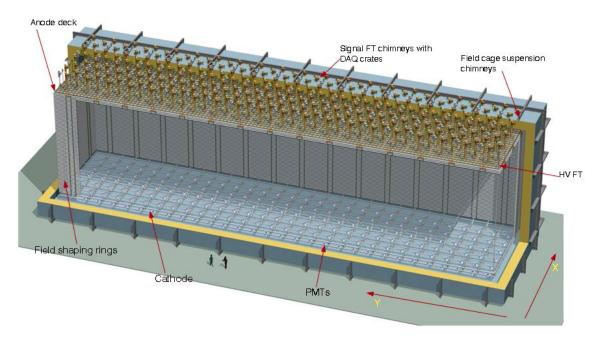
Figure 4.2. A DP module with cathode, PMTs, FC, and anode plane with SFT chimneys.
