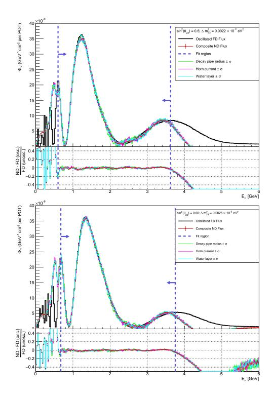
**Figure A.36.** Linear combinations of off-axis fluxes giving far-detector oscillated spectra for a range of oscillation parameters. The FD oscillated flux is shown in black, the target flux is shown in green, and the linearly combined flux obtained with the nominal beam MC is shown in red. Systematic effects due to  $1\ \sigma$  variations of the decay pipe radius (green), horn current (magenta) and horn cooling water layer thickness (teal) are shown.
