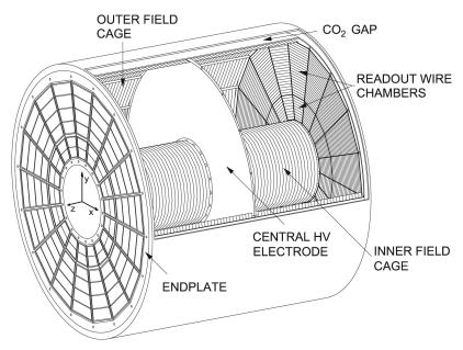
**Figure A.19**. Diagram of the ALICE TPC, from ref. [112]. The drift HV cathode is located at the center of the TPC, defining two drift volumes, each with 2.5 m of drift along the axis of the cylinder toward the endplate. The endplates are divided into 18 sectors, and each endplate holds 36 readout chambers.
