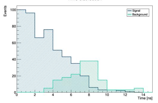
**Figure A.46**. Time difference between the neutrino interaction vertex time inside the  $1.0 \times 1.0 \times 1.0$  m<sup>3</sup> FV core of the 3DST and the earliest neutron-induced hit time. The neutron-induced hit leaves at least  $0.5 \, \text{MeV}$  in a single cube. The neutron-induced background hits arise from neutrons produced in neutrino interactions outside the FV.
