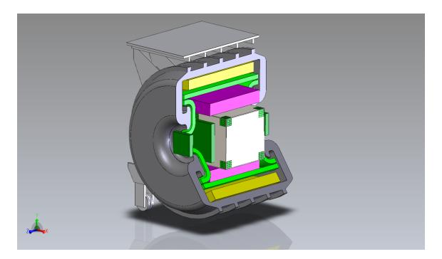
**Figure 5.6.** The SAND detector configuration with the 3DST inside the KLOE magnet. The drawing shows the 3DST in the center (white), TPCs (magenta), ECAL (green), magnet coil (yellow), and the return yoke (gray).
