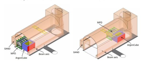
**Figure 1.13**. DUNE ND hall shown with component detectors all in the on-axis configuration (left) and with the LArTPC and MPD in an off-axis configuration (right). The beam monitor (SAND) is shown in position on the beam axis in both figures. The beam is shown entering the hall at the bottom traveling from right to left.
