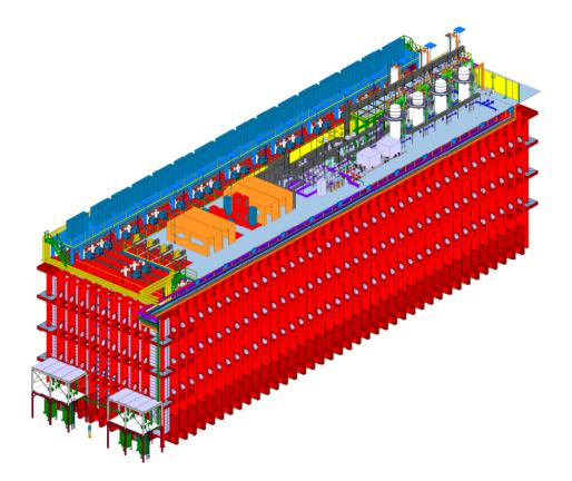
**Figure 3.1.** A 65.8 m (L) by 18.9 m (W) by 17.8 m (H) outer-dimension cryostat that houses a 10 kt FD module. A mezzanine (light blue) installed 2.3 m above the cryostat supports both detector and cryogenics instrumentation. At lower left, between the LAr recirculation pumps (green) installed on the cavern floor, the figure of a person indicates the scale.
