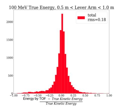
**Figure A.45**. Reconstructed neutron energy residual with lever arm larger than 0.5 m and smaller than 1 m for  $100 \,\text{MeV}$  for a  $2.4 \times 2.4 \times 2.0 \,\text{m}^3$  3DST detector.
