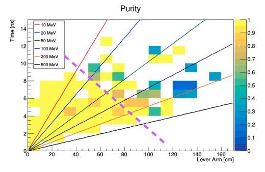
**Figure A.47**. Purity of the neutron-induced hit in the (time, lever arm) space. The dashed line corresponds to the cut required to select an almost 100% pure sample of signal neutrons. The solid lines are theoretical curves for neutrons with different kinetic energies. Note that this study was performed with a total volume of  $2\times2\times2$  m<sup>3</sup>. See text for details.
