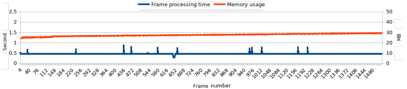
Figure 7. Original code base running on a tuned Ubuntu/Linux in a WCS. AVG energy consumption: 4.9J/frame.
