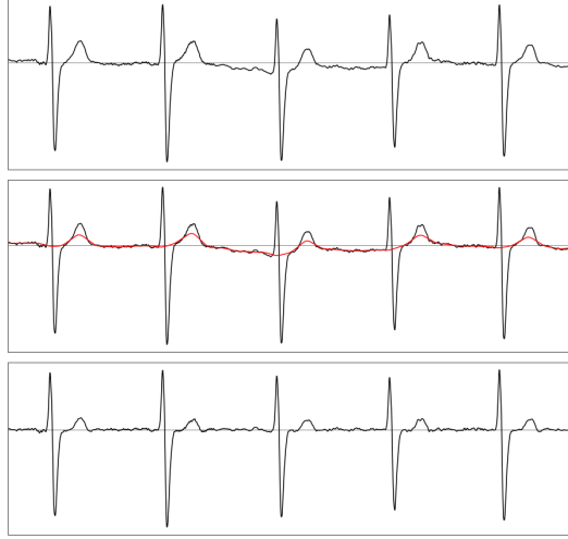
Fig. 6: top: original ECG signal. middle: ECG signal with estimated baseline drift (in red). bottom: ECG signal after removing baseline drift. (Note that the height of the T-wave is not preserved after filtering. This will not influence our results; we are interested in the preservation of short-term fluctuations rather than typical ECG components.)
