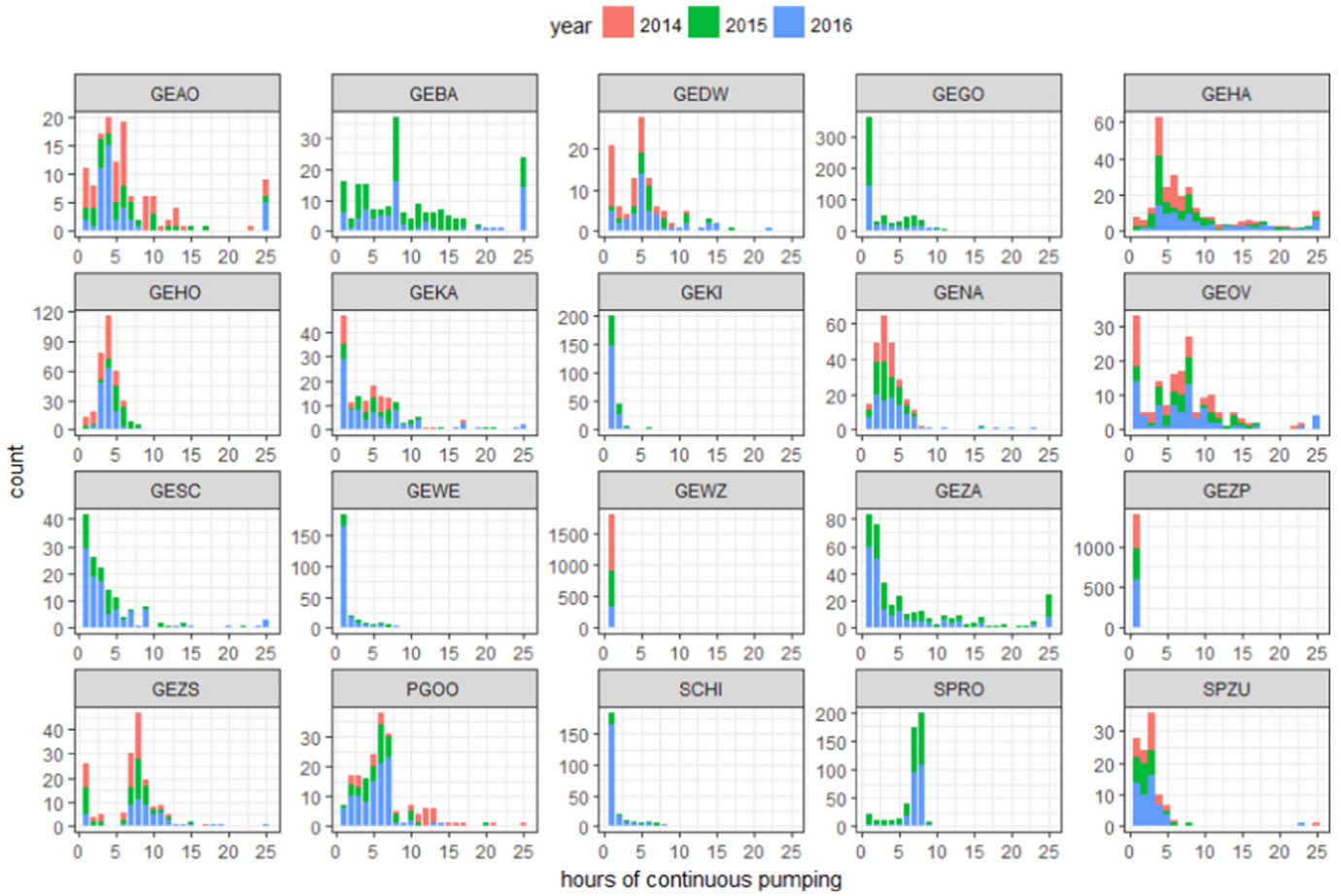
Fig. 3. Frequency distribution of single event duration of continuous pumping (bin width 1 h) per sampling location per year. Discharge data from water boards was used for sampled periods only.
