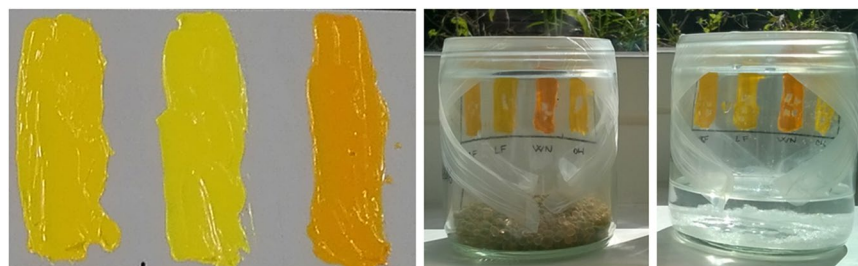
Figure 1. Paint layers and curing in dry and wet environment.
