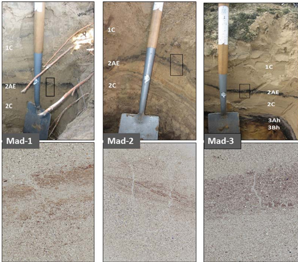
FIGURE 1.5.6 Three genetic types of micropodzols in field profile and thin section. (1) Monocyclic pedogenic micropodzol (left, Mad-1), clear ectorganic layer, overlying a mineral horizon with humic and albic properties. (2) Polycyclic pedogenic micropodzol (middle, Mad-2), the ectorganic layer is laminated. The soil formation was interrupted by short-lived sand drifting several times. The lower part of the older driftsand deposit is laminated, pointing to the result of a sequence of events; the colour differences are geogenic. (3) Geogenic micropodzol (right, Mad-3), showing a weakly developed Rhizomull with a sedimentary distribution pattern of organic particles. On the base of the humus form we can distinguish a discontinuous organic layer (decomposition of short-lived lichens/moss vegetation).
