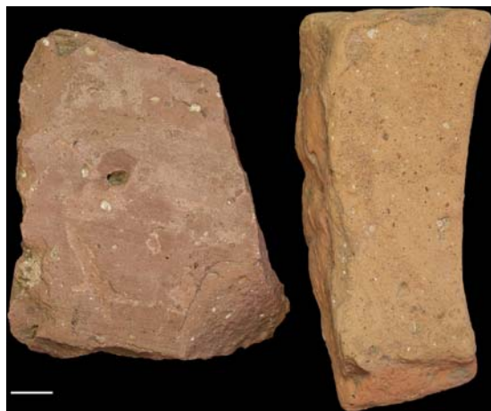
FIGURE 6.3.7 Fragments of tiles produced in the relics of the Roman tile-works close to mardel Kalefeld (length of the bar is 1 cm).
