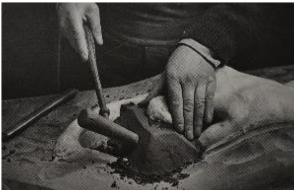
Fig. 4.25. The making of a false-core in sand with the use of a mallet. (from Baudry 2005, 279)
