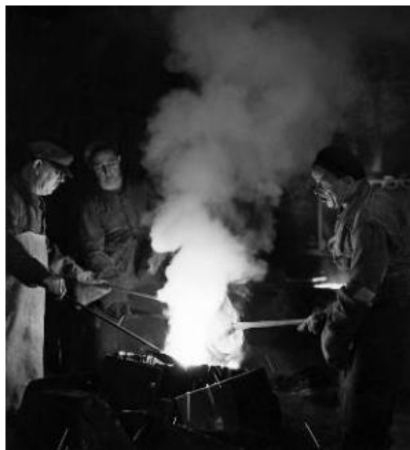
Fig. 4.50. Robert Doisneau, silver gelatine print, Paris, 1950. Pouring molten bronze into a mould, with the workman on the left protecting a riser hole by using a skimmer to prevent any dross from entering the mould. (image Doisneau estate)
