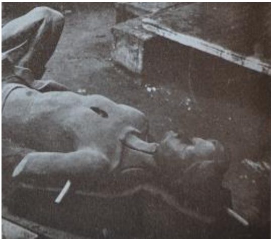
Fig. 4.39. Detail of the sand core for Malvina Hoffman's Brahman in meditation in the Rudier foundry (1934-36). In the neck are channels carved, creating reinforcing ribs in the interior of the bronze. (from Hoffman, 1936; 88. original by Clarence Buckingham Mitchell, Malvina Hoffman's son in law)
