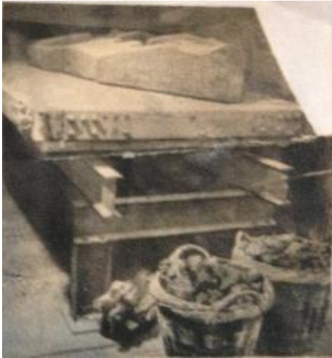
Fig. 4.47. Mould-pieces in the drying oven of the Rudier foundry. (between 1934-52) (image from an undated Dutch article called “ Hoe men bronzen beelden giet ” in the Malvina Hoffman papers, Box 15.2, Special Collections Getty Research Institute, Los Angeles.)
