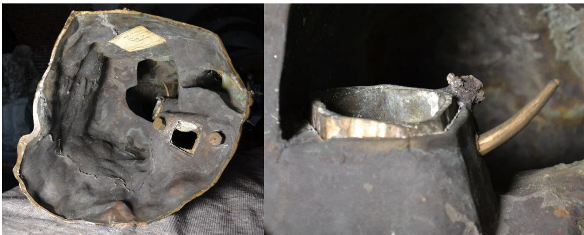
Fig. 4.63. The interior of the Brussels Petermann cast of the original size Thinker from 1899, illustrating the mechanical joining of the left leg.
