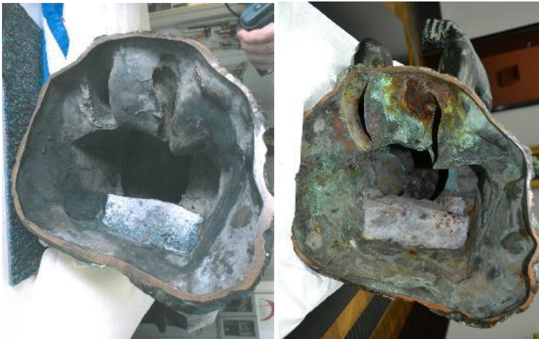
Fig. 4.96. Interior view of original size Thinkers cast by Eugène Rudier. On the left the Washington Thinker (1903) and on the right the Alte Nationalgalerie Thinker in Berlin (1905). Both display the early brick shaped counterweight, which is placed high up inside the back of base. (image left from the National Gallery of Art, Washington)
