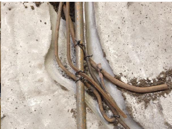
Figs. 4.34a & b. Iron armature consisting of round and square iron, in various diameters, suspended inside the drag mould. Images of piece-mould making in natural sand at the Bedi-Makky foundry in Brooklyn New York City, taken in May 2015.
