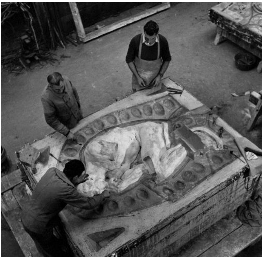
Fig. 4.28. Robert Doisneau, silver gelatine print, 1950. The monumental Thinker during moulding. The plaster foundry model in the drag mould with still a false-core visible around the ankle. The ovoid depressions are keys and the grooves visible between the keys and the pattern are runners. This foundry model is in line with the foundry models of the original size Thinker divided up in parts. Image taken by Robert Doisneau in the Alexis Rudier foundry in 1950, documenting the moulding and casting of a monumental Thinker . (image Doisneau estate)
