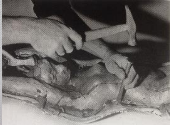
Fig. 4.54. The removal of runners by cutting with a chisel (from Baudry 2005, 282)
