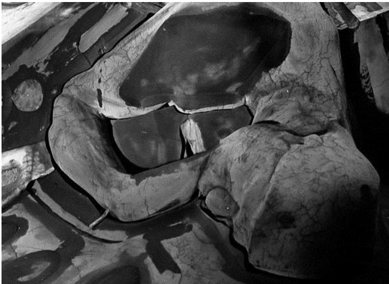
Fig. 4.43. Cracking of the core's surface. Detail of monumental Thinker during moulding. The core is already suspended inside the mould, resting on the core support irons. Note the gap between the core and the mould. The black stripes are the charcoal coating of the mould interior. Image taken by Robert Doisneau in the Alexis Rudier foundry in 1950 documenting the moulding and casting of a monumental Thinker . (image Doisneau estate)
