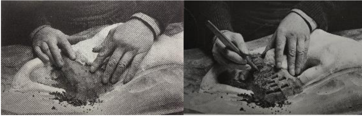
Fig. 4.24. First step in the making of a false-core in sand, with on the left the pressing by hand and on the right with a rammer ( fouloir ). (from Baudry 2005, 279)
