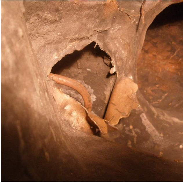
Fig. 4.44. Extensive flashing visible in the interior of the Geneva Thinker , also note the core-iron does is bent and does not extend beyond the flashing.
