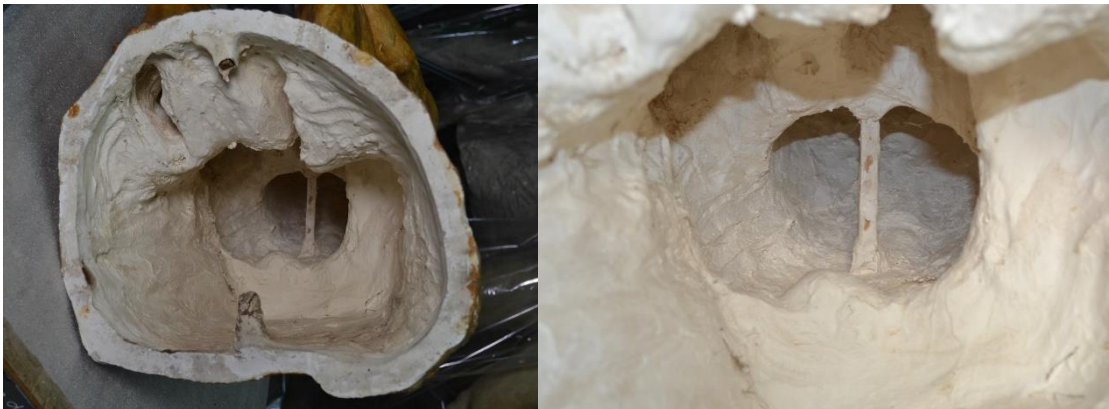
Fig. 4.13. A view of the underside of the base of foundry plaster S.2839, with remnants of the wooden cross and another wooden reinforcement deeper in the plaster visible.
