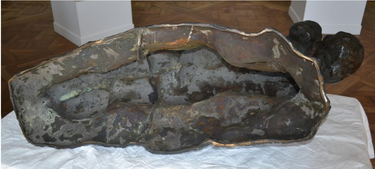
Fig. 4.60. Underside of Rodin's La Terre (Rodin Museum, Paris, S.623). A sand mould casting by E. Groult, dating from probably 1897, where two separate castings are joined in the middle by brazing.
