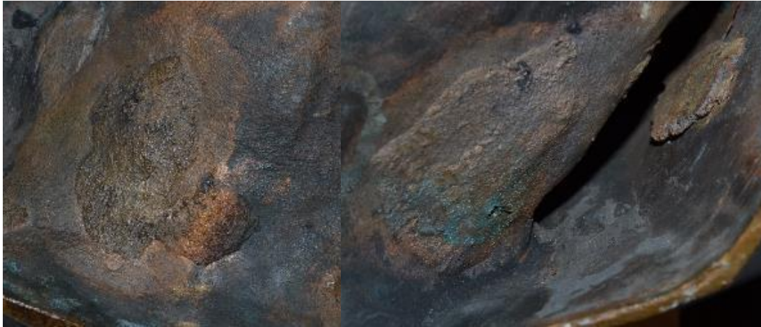
Fig. 4.62. Details of the interior surface of the Idylle illustrating two spots where the figures were joined by burning. The rough and slightly higher surface is where the metal fused. Also visible on the right image is a cast-on surface repair.
