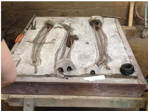
Figs. 4.34a & b. Iron armature consisting of round and square iron, in various diameters, suspended inside the drag mould. Images of piece-mould making in natural sand at the Bedi-Makky foundry in Brooklyn New York City, taken in May 2015.
