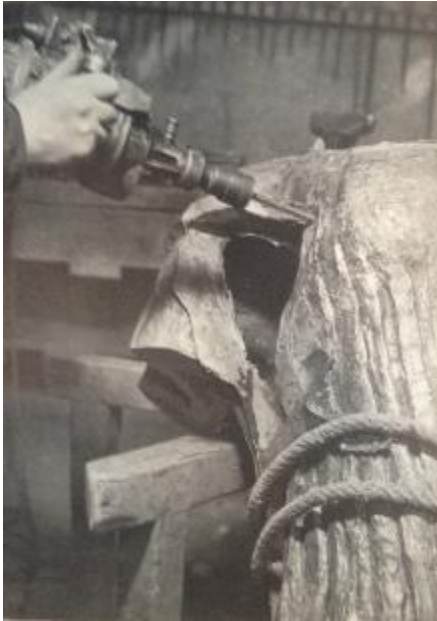
Fig. 4.65. Electric drill used at the Rudier foundry to drill holes for the mechanical joining of parts. (image 1936 or earlier) (from Hoffman 1939, 301)
