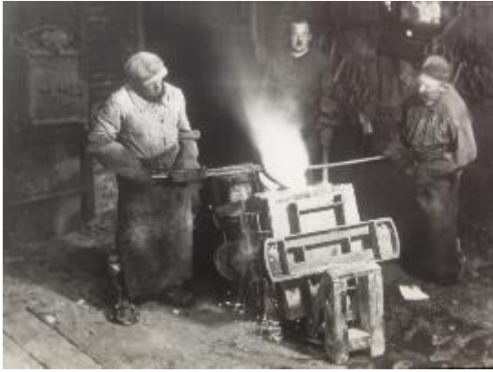
Fig. 4.48. Pouring the molten bronze into the mould in the Alexis Rudier foundry, Paris (1934-36) (from Hoffman, 1936, 89, original probably by C. Mitchell)
