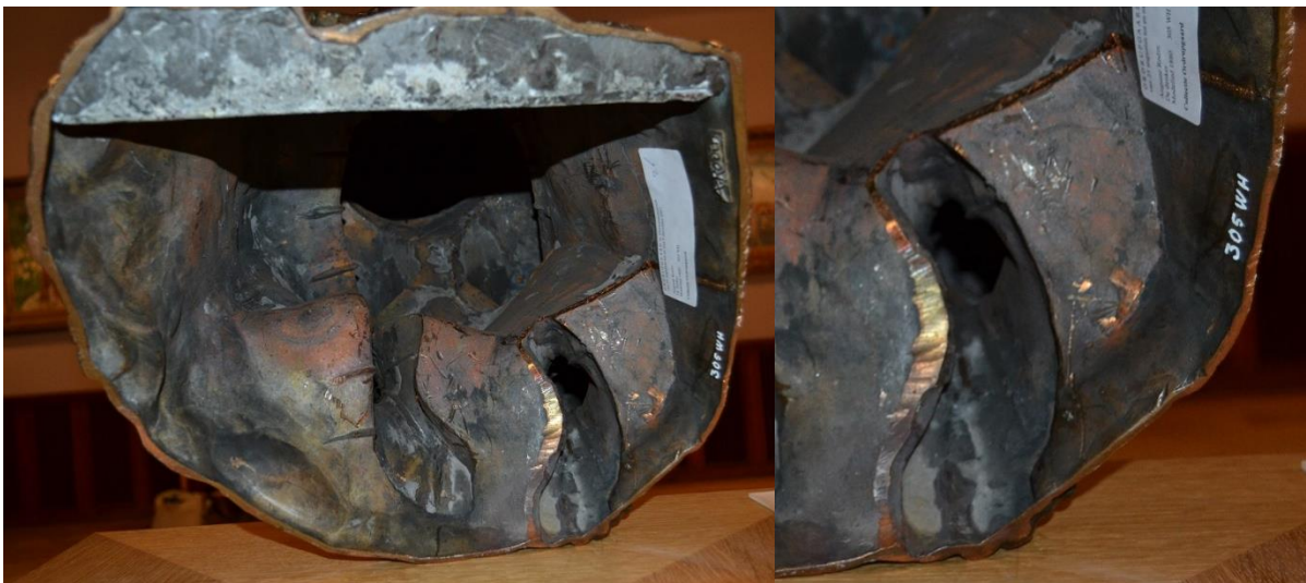
Figs. 4.45a & b. Underside of the Ordrupgård Thinker with in the lower right corner the finished shiny flashing lines visible.
