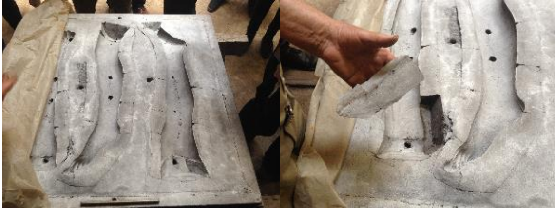
Fig. 4.29. One half of a piece-mould without the core at the Bedi-Makky foundry of Brooklyn. On the right a false-core is removed to illustrate the modular nature of the mould.
