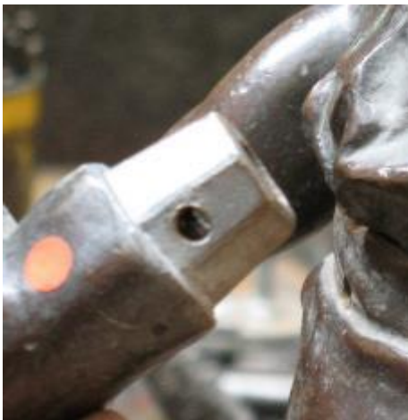
Fig. 4.4. Detail of a pattern at the Chardon & Petit Fils foundry in Paris, illustrating the male part of a sleeve or Roman joint. (image Jane Bassett, Getty Conservation Institute, Los Angeles)
