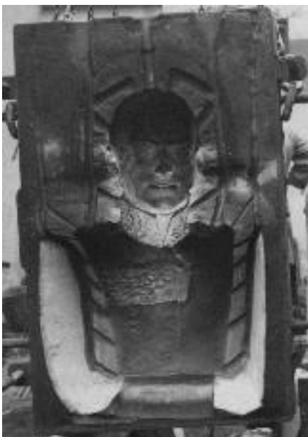
Fig. 4.46. The cope of a bust with the carved gating system, note the space for the lantern in the top of the mould. (image taken in an unknown foundry, probably French first half twentieth century, image private collection)
