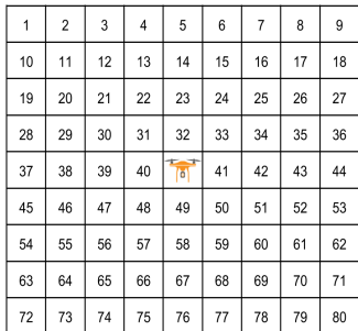
(a) Feature design 1 - centered around the robot with a map of size 9 \times 9 . This is all-grid uniform feature design.
