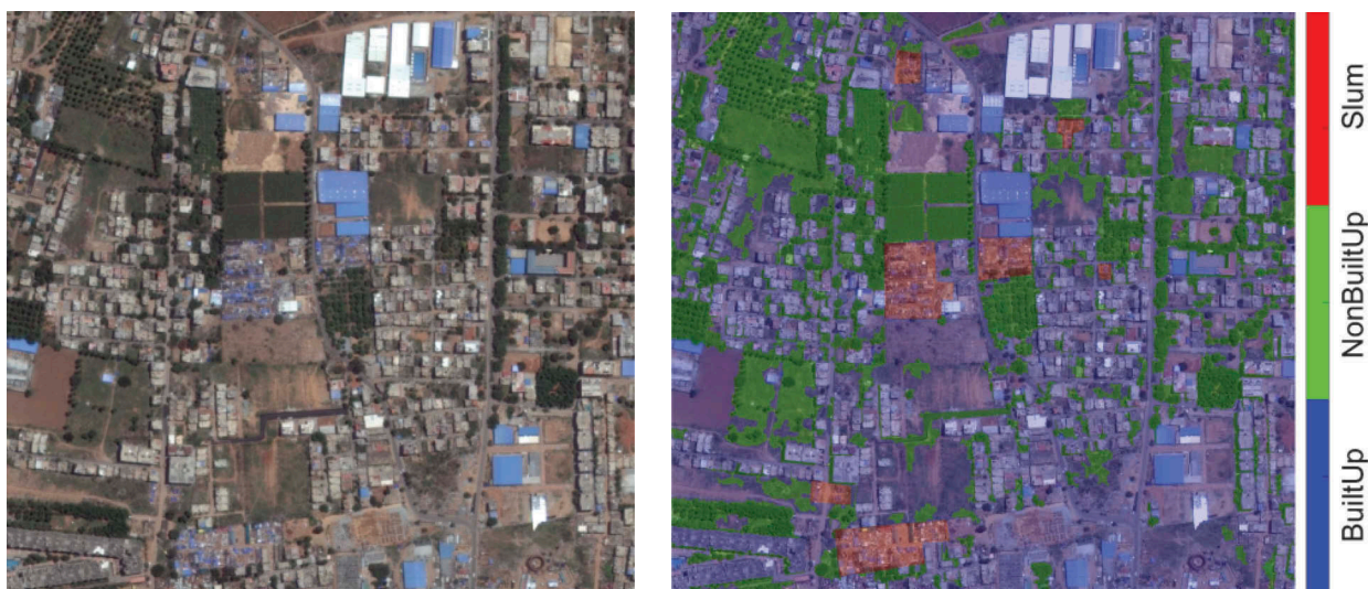
Figure 6. The second of the selected Bangalore ROIs. Left: original image and Right: overlaid ground truth for slums, non built-up (vegetation) and the remaining areas (built-up).
