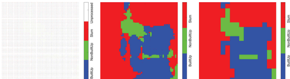
Figure A3. Pixel-level segmentation of Bangalore ROI2 (zoom). Left: Initial class label via classification of a tile with size 40m centred around these pixels; Middle: Assignment of labels to all unprocessed pixels with window size 22; Right: Final segmentation – all pixels within each window of size M = 30 get the majority label.
