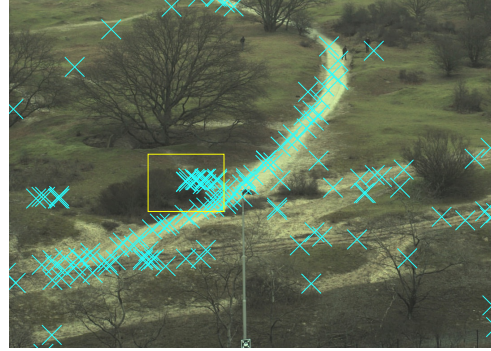
Figure 3: Particle belief: the yellow rectangle shows a pixel box and the particles it covers.
