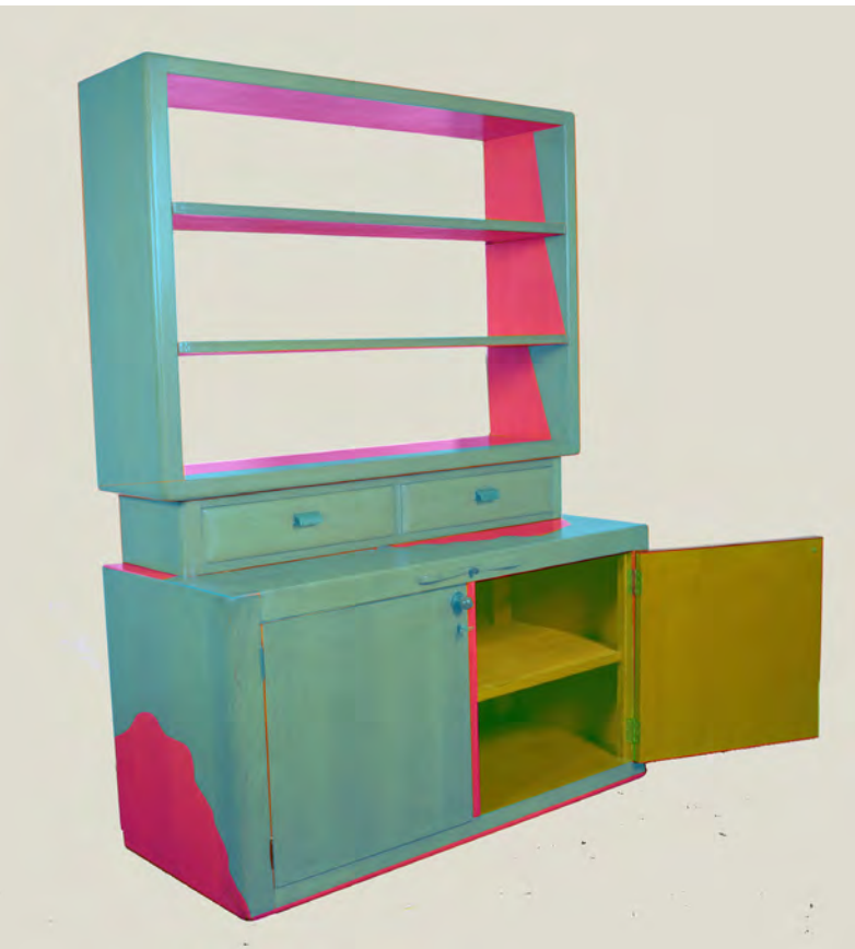
Figure 5 Three stages of degradation of the monochrome orange dye are set out: green: the orange colour has hardly changed, pink: these parts were often located in the shade and are still quite orange, blue: no orange colour is left; a slight orange shade can be recognised.
