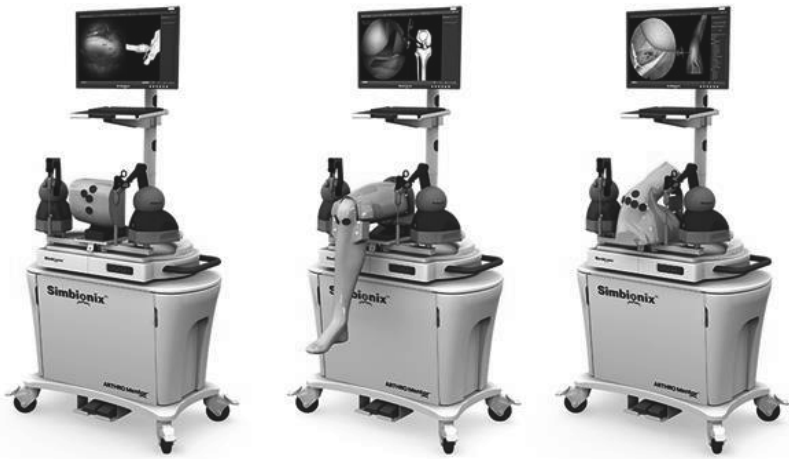
Figure 6: ARTHRO Mentor™ VR simulators for hip, knee and shoulder arthroscopy (Reprinted with permission from www.simbionix.com )
