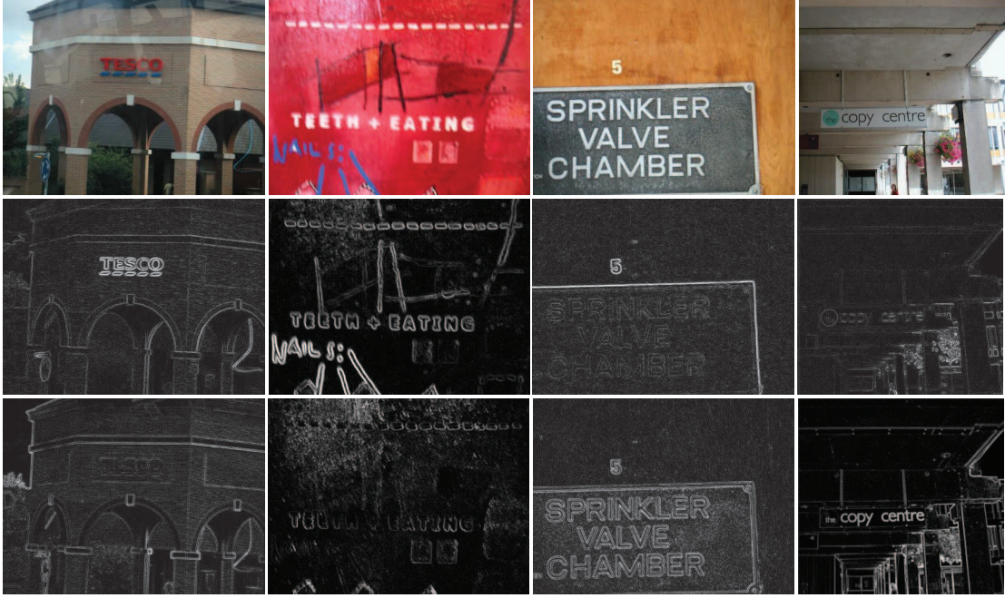
Figure 12: Saliency map samples: Original images, color saliency and curvature saliency (top to down order). It is shown that text edges are detected better with color saliency for the first two images whereas curvature saliency works better for the last two images.
