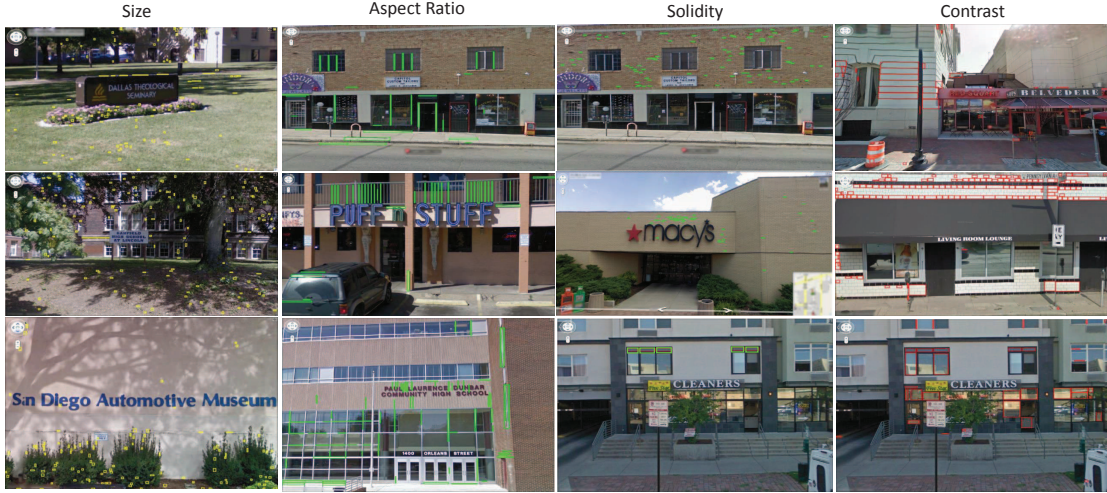
Figure 15: Samples for character candidate filtering. The green, red and yellow (different colors are used to highlight boxes) boxes represent filtered character candidates after corresponding filtering condition is applied (i.e. size, aspect ratio, solidity and contrast).
