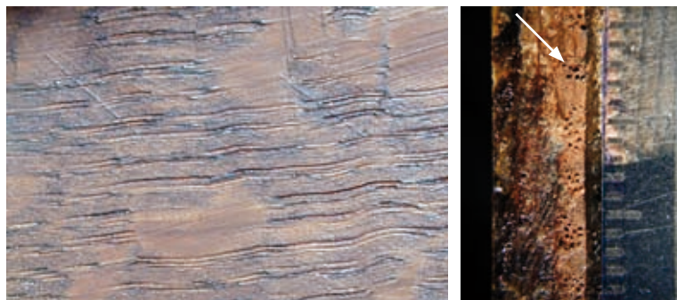
Fig. 5.6 Microscope detail of reverse of Aert van der Neer showing deep channels of the oak panel ( left ). Detail of the transverse section (end grain) showing chalk ground that preferentially fills the large cells of early wood ( right ).
