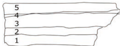
Fig. 3.A.6 Schematic layer build-up of the “healthy” black area (B). (1) ground layer (0-25 \mu\text{m} ). (2) brown underpaint layer (7-25 \mu\text{m} ). (3) flesh tone (25 \mu\text{m} ). (4) thin brown layer (5 \mu\text{m} ). (5) bone black layer (15-20 \mu\text{m} ).
