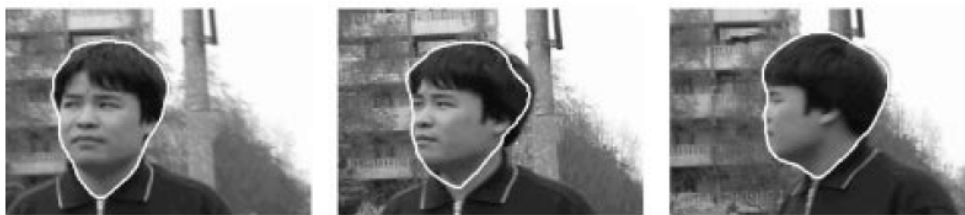
Figure 2.6: An example of active contour-based tracking. Three frames are shown with the active contour in white. From [Nguyen et al., 2002].
