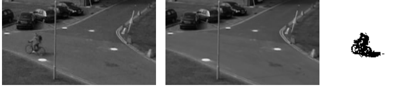
Figure 2.4: Example of the use of background modelling. On the left a frame from the input sequence is shown. The center image shows the learned background. On the right the segmented foreground is shown.
