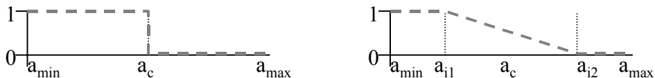
Figure 7.18. The density of the class distribution for (a) a strict class boundary that comes with an orthogonal concept and (b) a non-strict class boundary that belongs to a linear class boundary.
