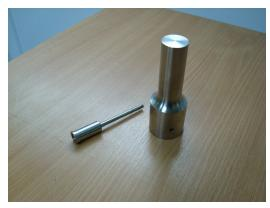
Fig: A3.10. Low and High powered piezoelectric transducer.
