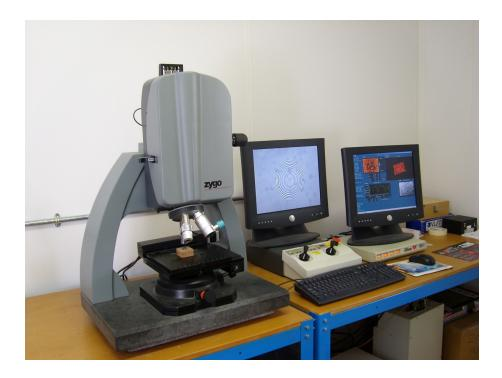
Fig: A3.4 ZYGO Surface scanning microscopy
