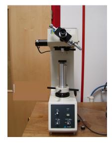
Fig: A3.1 Buehler Vickers Indent generating device
