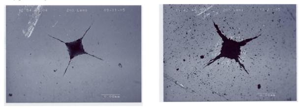
(a) (b) Fig: 3.49 (a) & (b) Eroded Indent after 30 and 60 minutes.
