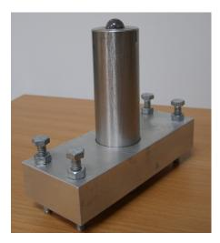
Fig: A3.11. Specimen holders' for cavitation experiments.
