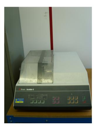
Fig: A3.12. Cutting machine for specimen dicing.
