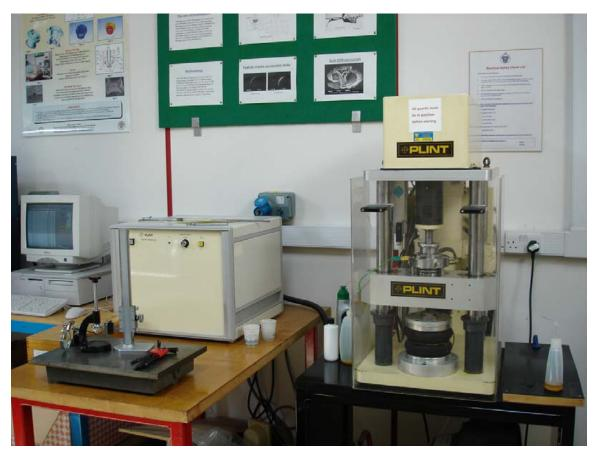
Fig: 2.9. Rolling contact fatigue test facility.
