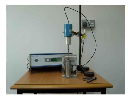
Fig: A3.8. Cavitation erosion test setup.
