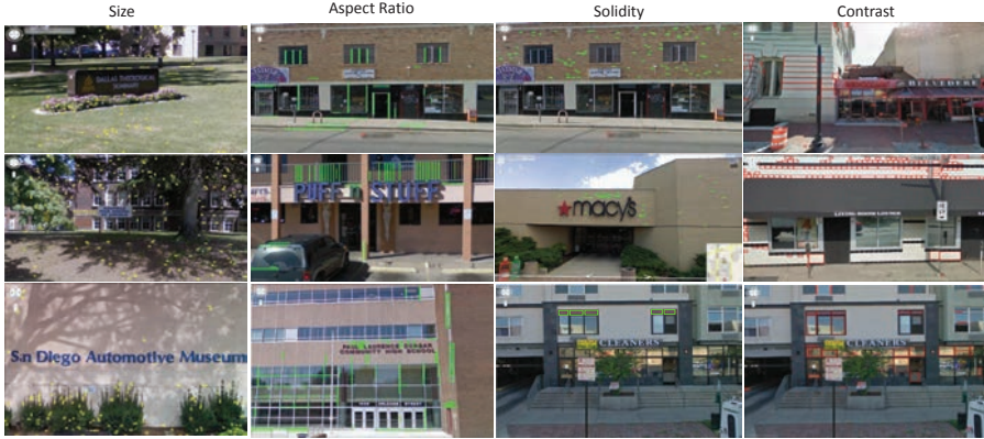
Figure 5.5: Samples for character candidate filtering. The green, red and yellow (different colors are used to highlight boxes) boxes represent filtered character candidates after corresponding filtering condition is applied (i.e. size, aspect ratio, solidity and contrast).
