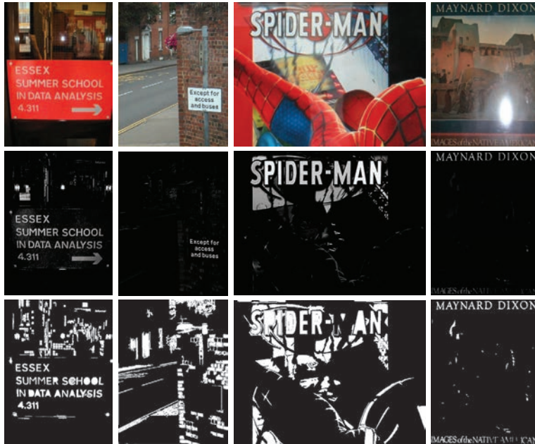
Figure 5.3: Original images (up), text saliency (middle) and MSER character detections (down) obtained. Text saliency method is robust against changes in text size and noise while MSER detects characters at image boundaries.
