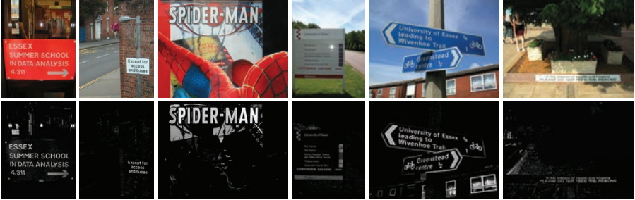
Figure 4.6: Original images and text saliency maps obtained. Most of the background regions are filtered out while text regions are preserved by the proposed method. The proposed method is robust against photometric changes e.g., shadow and highlights, text size, style and orientation.
