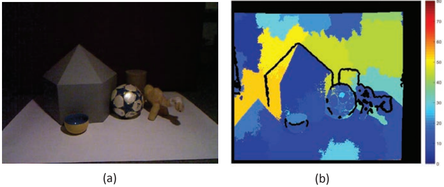
Figure 2.1: (Best viewed in color) (a) An image sample taken from [8]. (b) Image surface segments produced by the mean-shift algorithm and their individual angular errors. The color represents the angular error of each image surface segment. The corresponding angular error for each color is at the colorbar next to each plot. Dark blue regions represent smaller angular errors whereas dark red regions represent larger angular errors. The figure illustrates that curved (such as ball and bowl) and less textured (such as table and toy castle) image surface segments have lower LSP estimation errors. Moreover, regions with shadows or highlights have difficulties to estimate LSP.
