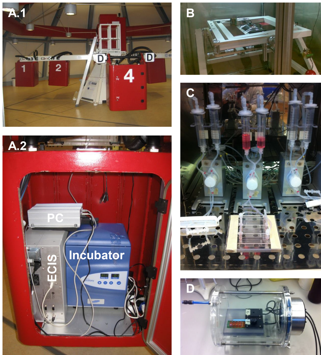
Fig 1. Experimental set-ups. A.1) Large Diameter Centrifuge (LDC) with outer gondolas for application of hyper-gravity and the central gondola for rotational controls. A.2) Measurement set-up for quantification of endothelial characteristics in one of the outer gondolas. The set-up consisted of ECIS system, PC and incubator. B) Random Positioning Machine (RPM) for simulation of near weightlessness. C) Pump-system for application of fluid shear stress. D) Custom made pressure vessel for exertion of hydrostatic pressure.
