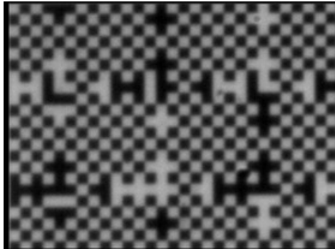
Figure 17: A RASNIK mask image projected onto a sensor. The code lines that replace the checkerboard pattern every ten lines are clearly visible.
