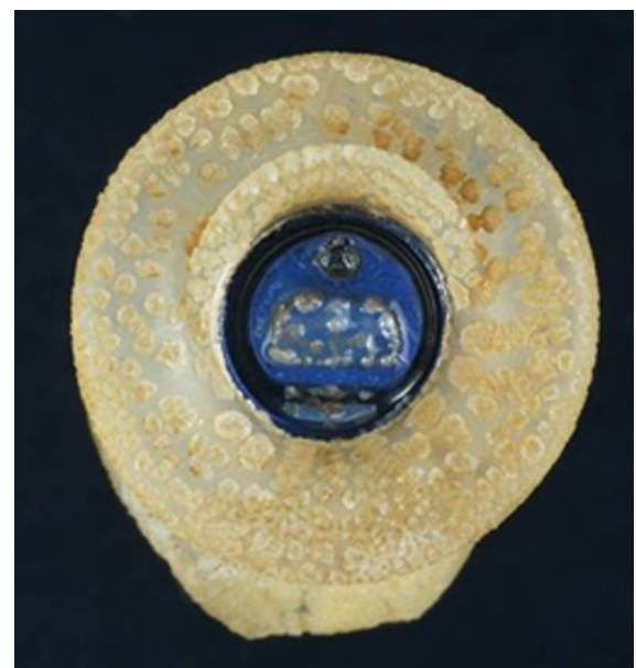
FIGURE 2. Macroscopic image of a Provox ActiValve, which was 364 days in situ, illustrating the amount of biofilm on the silicone material and on the fluoroplastic valve.
