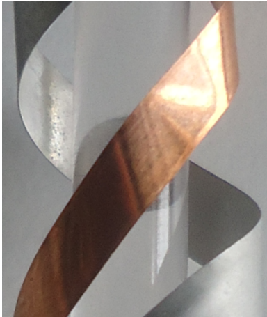
(a) Picture of the sample. Copper and cadmium foils are wrapped around a plastic rod.
