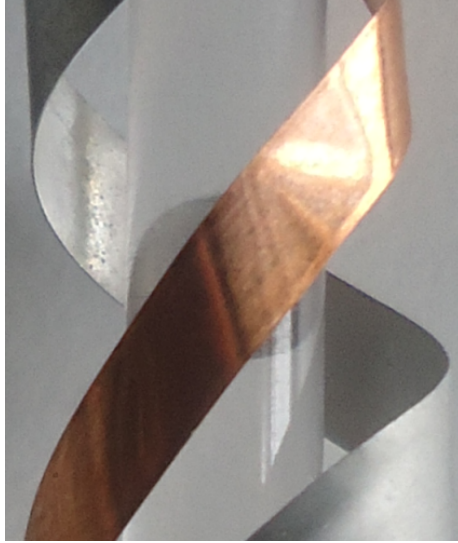
Figure 6.3: Picture of the sample used for the color CT proof of principle. Copper and cadmium foils are wrapped around a plastic rod.
