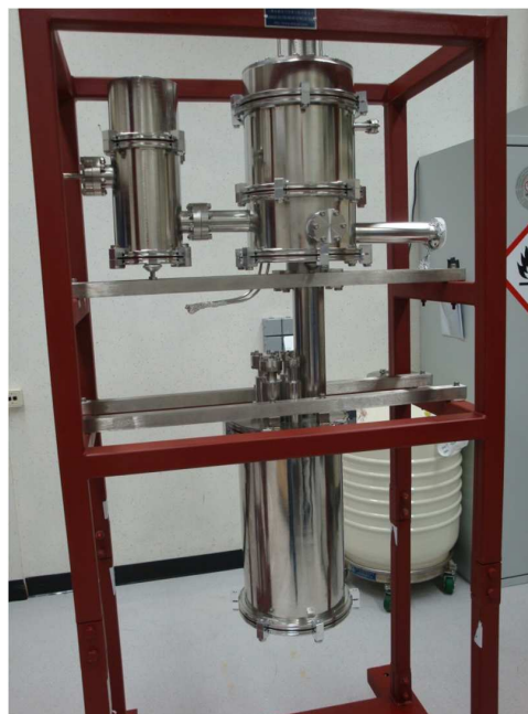
Figure 8. Cryostat of the dual phase xenon TPC under construction at Nikhef. The detector will be built in the bottom vessel while the top vessels will house the cooling system and the heat exchanger of the gas recirculation.
