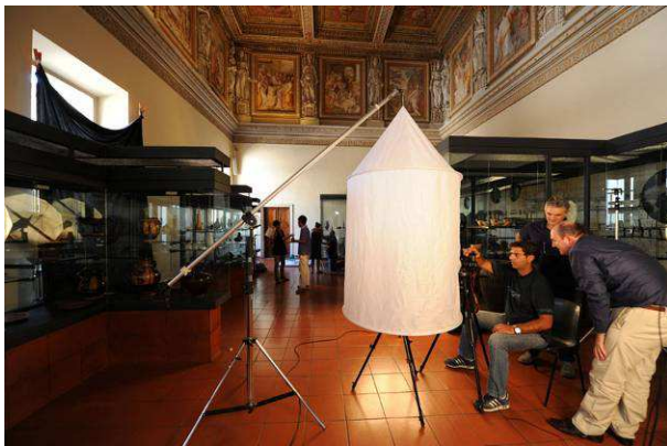
Figure 4: Objects digital photographic acquisition in Vatican Museums with turning table and a white tent
