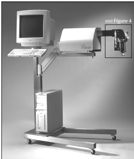
Figure 3. Commercialised RCM, the Vivascope® 1000.
