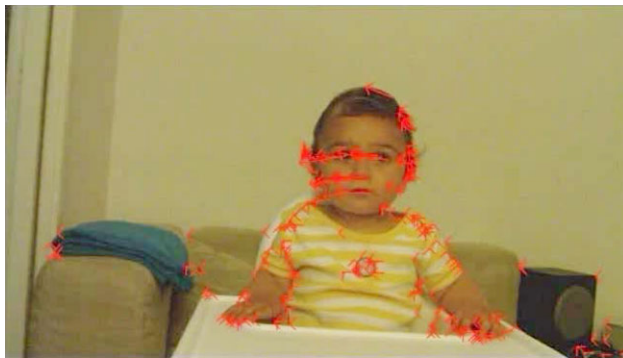
Fig. 4 Example of the optical flow vectors obtained in a frame using the pyramidal implementation of the Lucas and Kanade algorithm. Optical flow vectors are represented as red arrows in the picture
