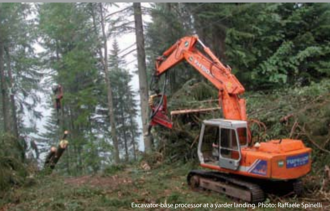
1500 m span tower yarder, processor and biomass recovery operation. Photo: Raffaele Spinelli
