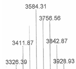
Figure 16. Part of the MALDI-ToF mass spectra (linear mode) of polymer obtained with [\{\text{Rh}^{\text{I}}(1,5\text{-cyclooctadiene})(\mu\text{-Cl})\}_2] in the presence of methanol.
