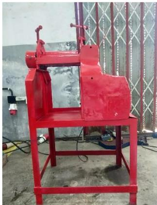
**Gambar 4.** Mesin Roll Iratan Bambu
