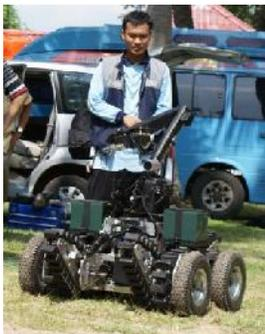
**Gambar 1** Mobil robot penjinak bom (Morolipi V1)
