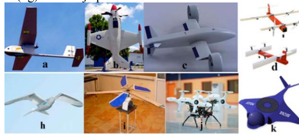
Slika 3. Neki važniji tipovi \mu UAVs, (a) HTOL, (b) VTOL, (c) tilt-rotor, (d) tilt-wing, (h) ornithopter, (i) ornicopter, (j) cyclocopter, and (k) unconventional UAV, [8].
