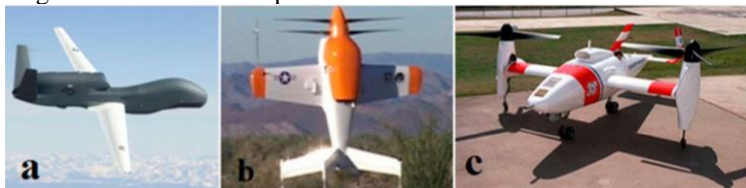
Slika 2. Neki važniji tipovi UAV dronova: (a) HTOL, (b) VTOL, (c) tilt-rotor UAV, [8]. Figure 2. Some important UAV tipe of drones:(a)HTOL, (b) VTOL, (c)tilt-rotor UAV,[8].
