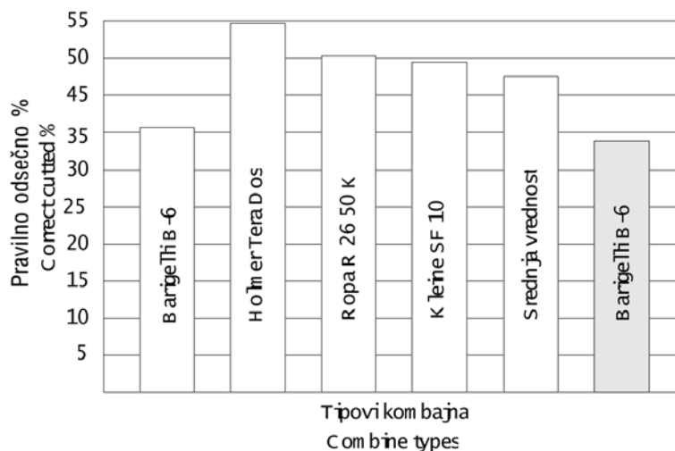
Sl. 2. Uporedni prikaz rezultata klase "pravilno odsečeno" Fig. 2. Results comparative review in class quality "correctly cut" of tested combines
