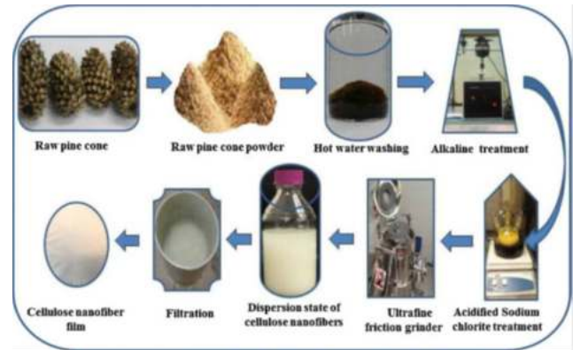
FIGURE 21. Schematic view of production of nanocellulose from pinecone biomass using chemical and mechanical treatments [74].
