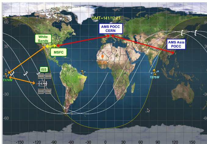
Fig. 32. World map showing the location of the ISS and the flow of AMS data on May 20, 2020 (day of year 141) at 12:21 GMT including the radio links (orange) from the ISS to the T174 W TDRS satellite and from T174 W to the White Sands ground terminal, the NASA internal network (yellow) connecting White Sands to the Marshall Space Flight Center (MSFC), and the Internet connection (red) from MSFC to the AMS POCC at CERN. The AMS data are re-transmitted over the Internet to the AMS Asia POCC in Taiwan. The ground track of the ISS for three orbits is indicated (white sinusoidal curves). The locations of the other two TDRS satellites active on this ISS orbit are shown (T041 W, T275 W). The day–night boundary is also indicated (dark yellow boundary of dark and light regions). The “staple” shapes along the orbital ground track indicate the location of the ISS where the Sun will rise and set. Latitude and longitude are indicated by the grid pattern.
