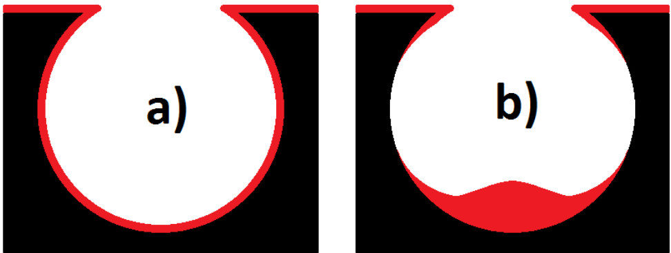
Figure 2.3: Comparison between a) conformal growth, and b) non conformal growth. Conformal films are favorable for applications where uniform coverage is needed to prevent short circuits or other nonuniform behavior, whereas non conformal, or directional growth is preferred when only one side of a feature needs covering, such as in lift-off procedures.
