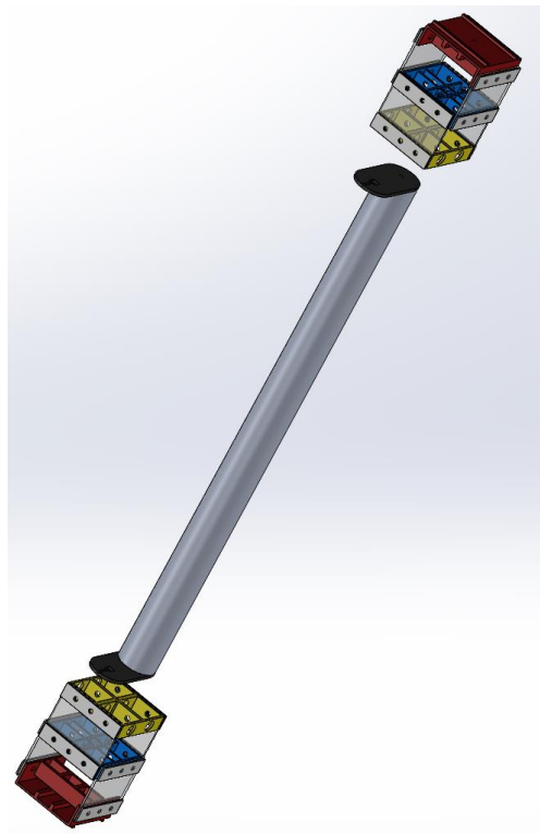
Figure 15: A 3D-rendering of the cylinder leaf spring configuration used.
