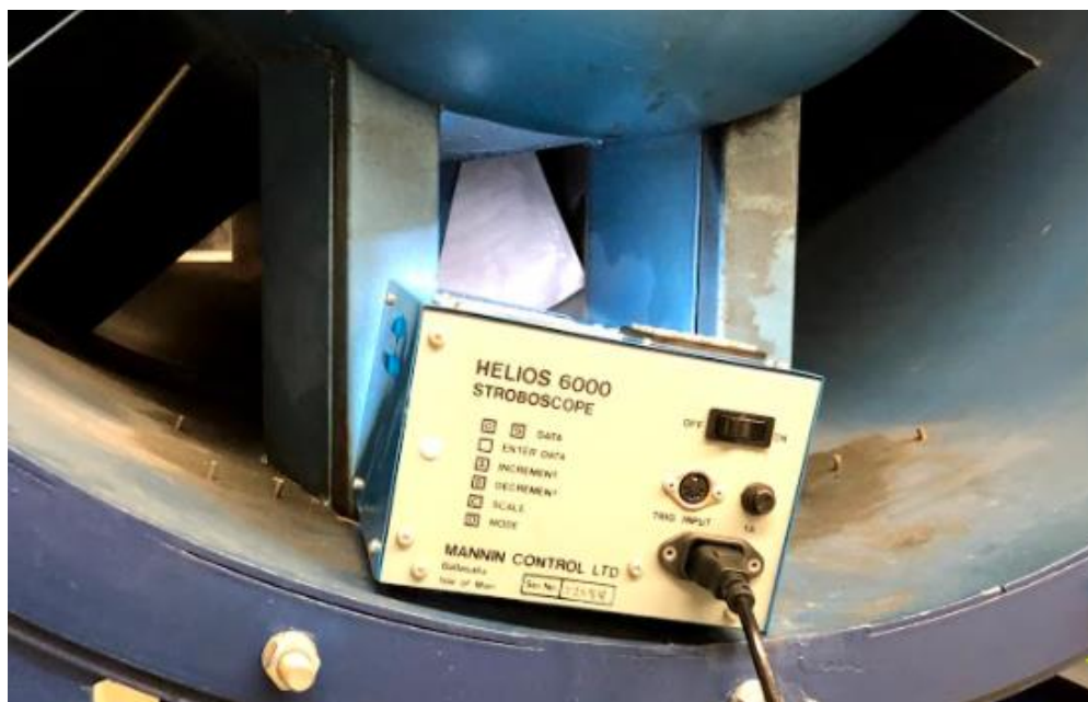
Figure 10: The stroboscope capturing one blade pass during wind tunnel operation.
