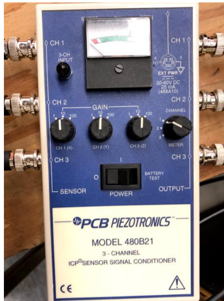
Figure 22: PCB signal conditioner used to convert accelerometer signal.
