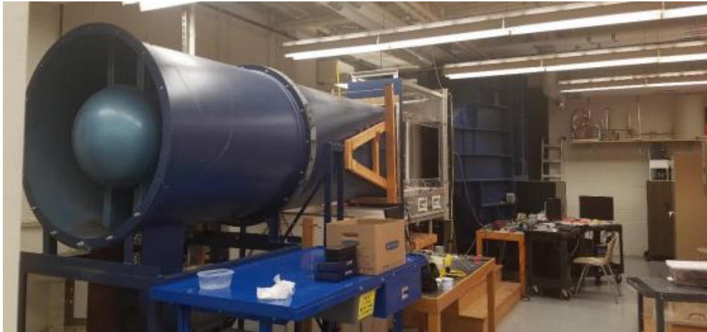
Figure 7: Open return subsonic wind tunnel.
