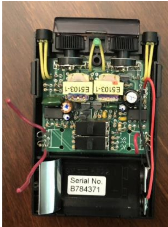
Figure 3.3: Contraction wire cut to create open circuit (photo by Pablo Valenzuela)
