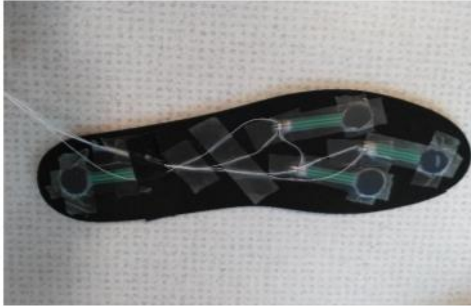
Figure 2.8: Insole containing the four FSRs (Photo by Prem)
