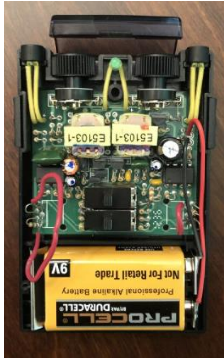
Figure 3.2: EMS circuit connected with 0 resistance wire (photo by Pablo Valenzuela)
