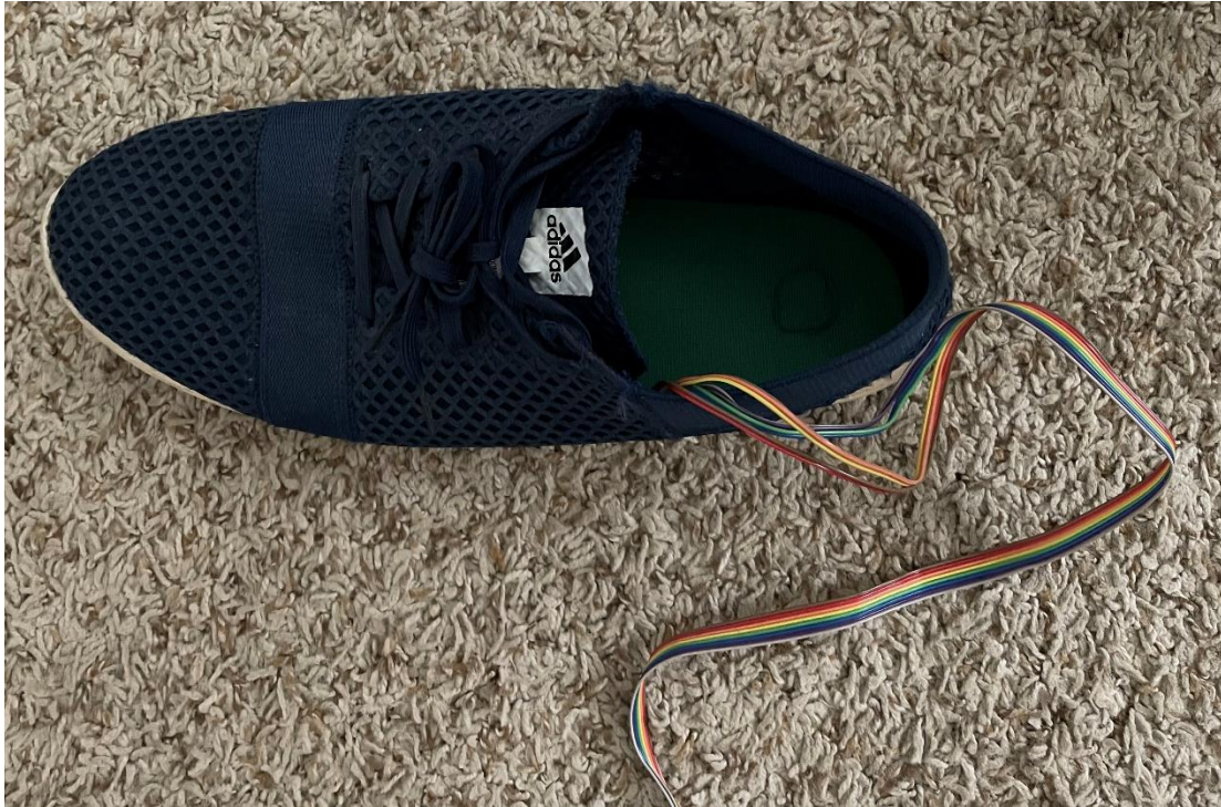
Figure 3.7: FSRs shoe insert placement (photo by Pablo Valenzuela)
